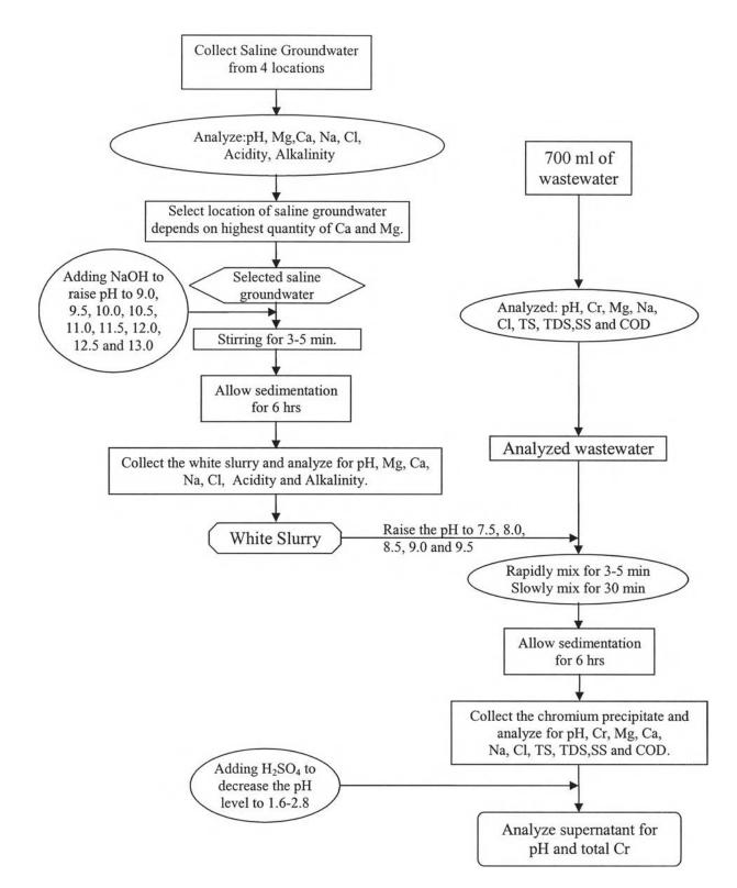
Figure 3.1 Flowchart of methodology of chromium recovery from tanning wastewater.
