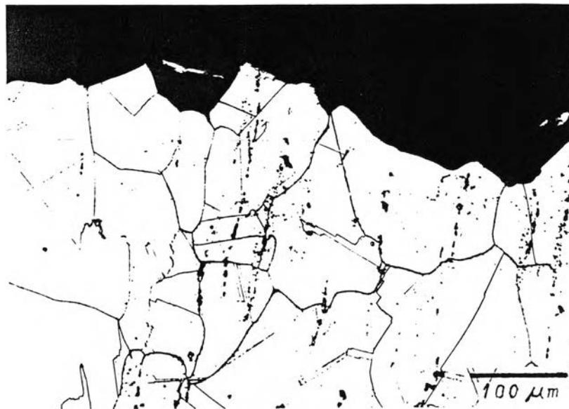
Figure 4.10 As Fracture Profile Line at Fracture Surface 50 X
