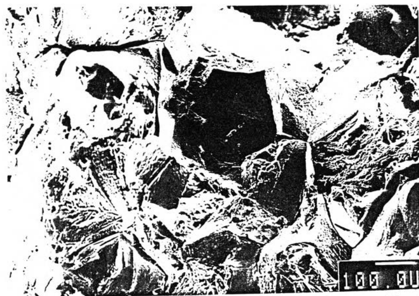
Figure 4.29 As Fracture Initiated Intergranularly from Fatigue Test in SEM
