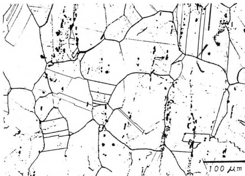
Figure 4.11 As Low Deformation Microstructure of Primary Creep Stage 50 X
