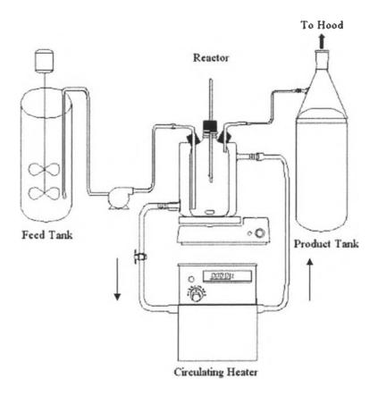
Figure 3.1 Continuous admicellar polymerization system.
