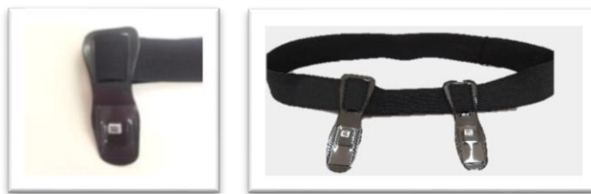
Figure 3.3 Eye lens dosimeter attached to the head band
