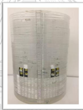
Figure 3.1 Cylindrical head phantom with eight nanoDots inserted and attached
