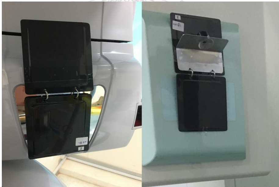
Figure 2 Two pieces of 1.0 mm thick copper filters were attached to the CBCT machine (Veraviewepocs 3D R100 and 3D Accuitomo 170)
