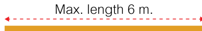
Figure 48 The maximum length for the panel is 6 m due to restrictions in transportation law.
