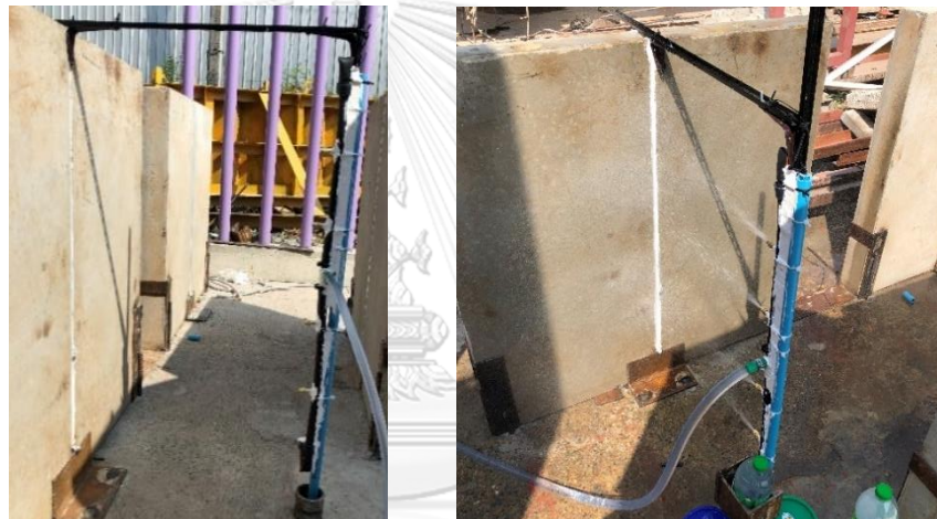
Figure 12 The equipment used in the water spray test and the installation before and during the test.
