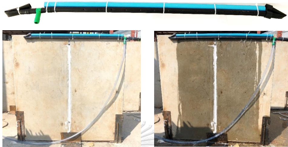
Figure 11 The equipment used in the surface flow test and the installation to the test module before and during the test.
