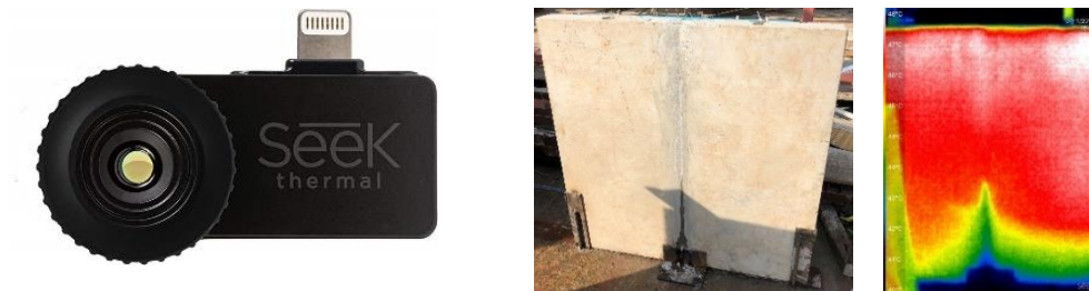
Figure 14 The Seek thermal Compact equipment and the example of the collected thermal image.
