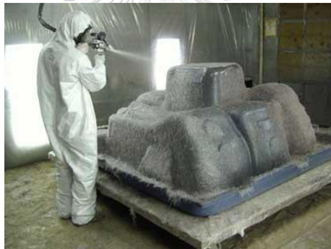
Figure 2-15 Production process of fiberglass by spraying
