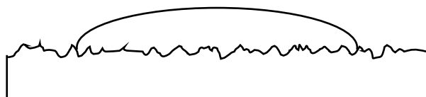
Figure 2.6 Good wetting by an adhesive spreading over a surface
