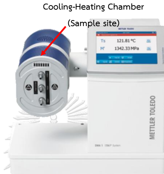
Figure 13 Dynamic mechanical analyzer (DMA)
