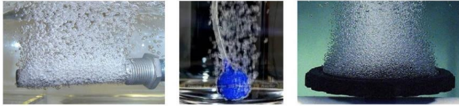
Figure 2.10 Bubbles creation by diffusers in millimeter range
