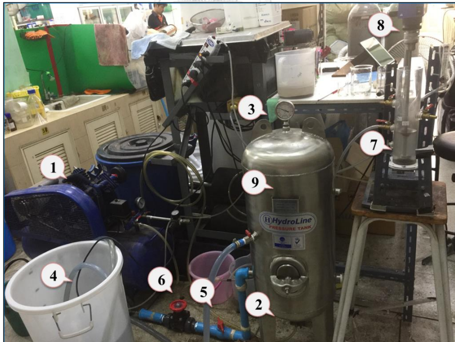
Figure 3.4 Experimental set-up of stirring with dissolved air flotation (DAF)
