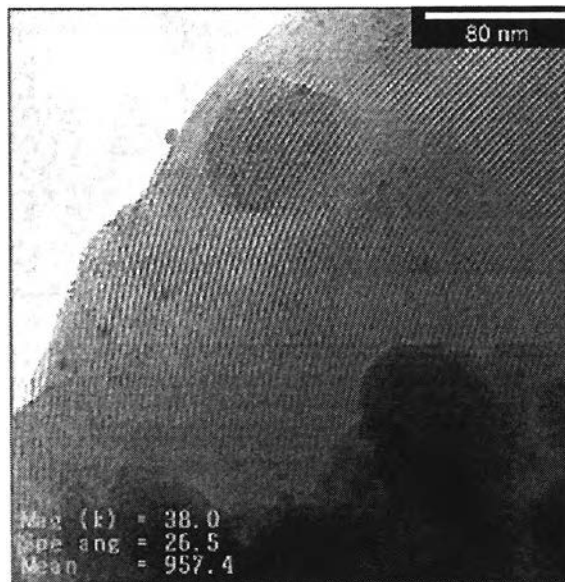
Figure 1.2 TEM micrograph of MCM-41, showing the slightly curved uniform mesopores running through the silica matrix [20].
