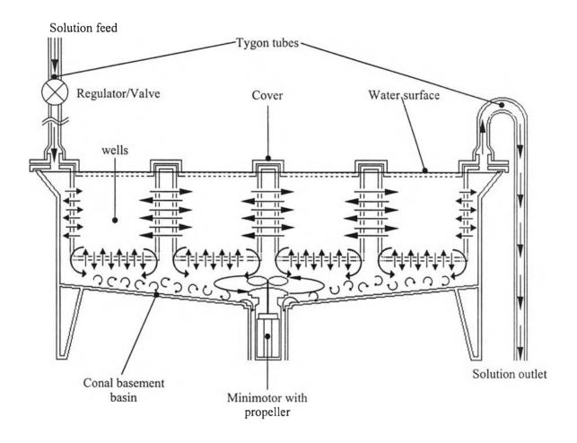
Fig. 5.1 Schematic diagram of proposed anti-cannibalism toxicity test container. Straight and curve arrows indicate water circulation, small circular arrows represent sediment transport.
