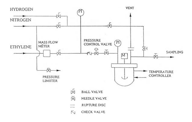
Figure 3.1 Schematic diagram of polymerization reactor.
