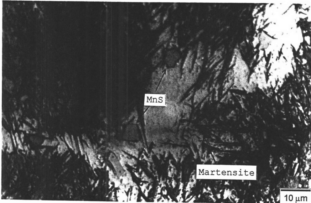
Fig.4-10 Sulfides precipitates of specimen that solidified with cooling rate of 3°C/s to 896°C and then quenched.
