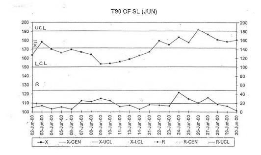
Figure 4.1 : The Control Chart for Melamine Compound's Curing Time of the Company in June 2000.
