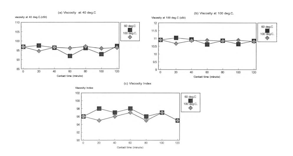
Fig. 5.14 Compositions of 500 SN after percolation process at various contact time and different temperature, 60 C and 100 C.
