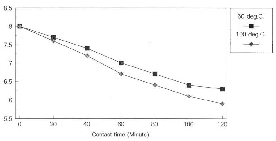
Fig. 5.7 Sulphur content of 450 SN after percolation process at various contact time and different temperature, 60 C. and 100 C..
