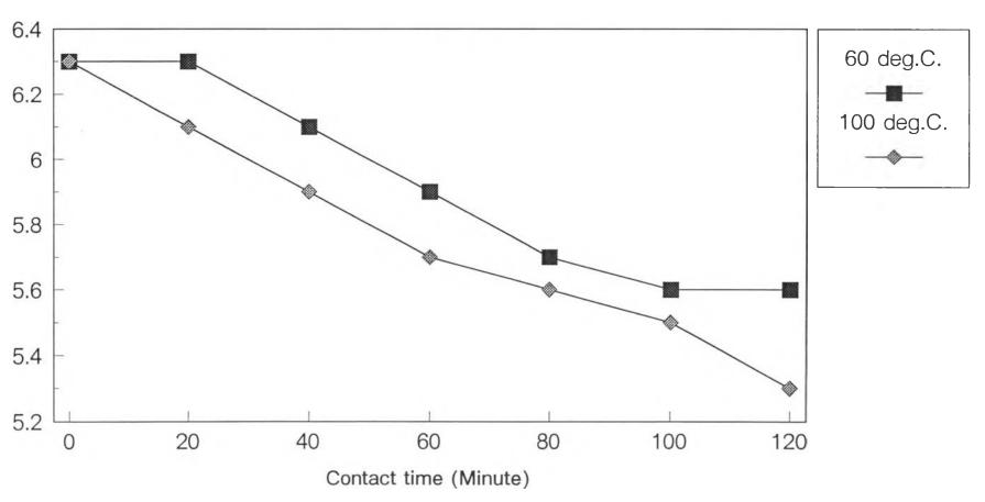
Fig. 5.12 Sulphur content of 500 SN after percolation process at various contact time and different temperature, 60 C and 100 C.
