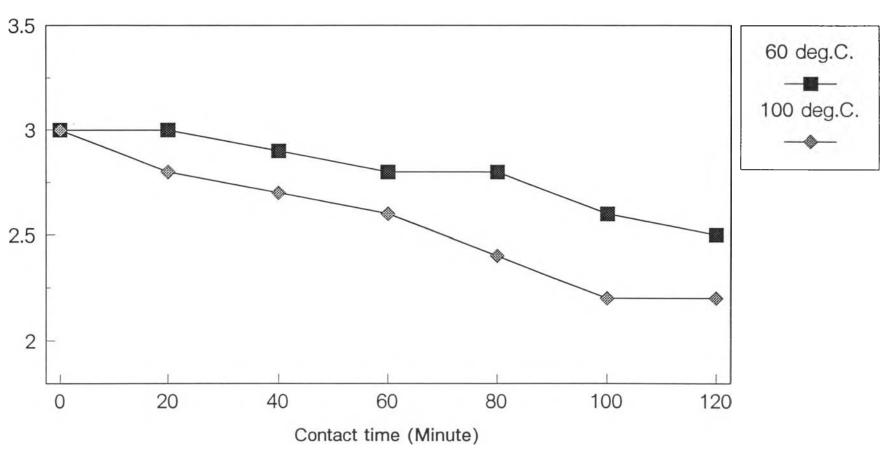
Fig. 5.2 Sulphur content of 150 SN after percolation process at various contact time and different temperature 60 C. and 100 C.
