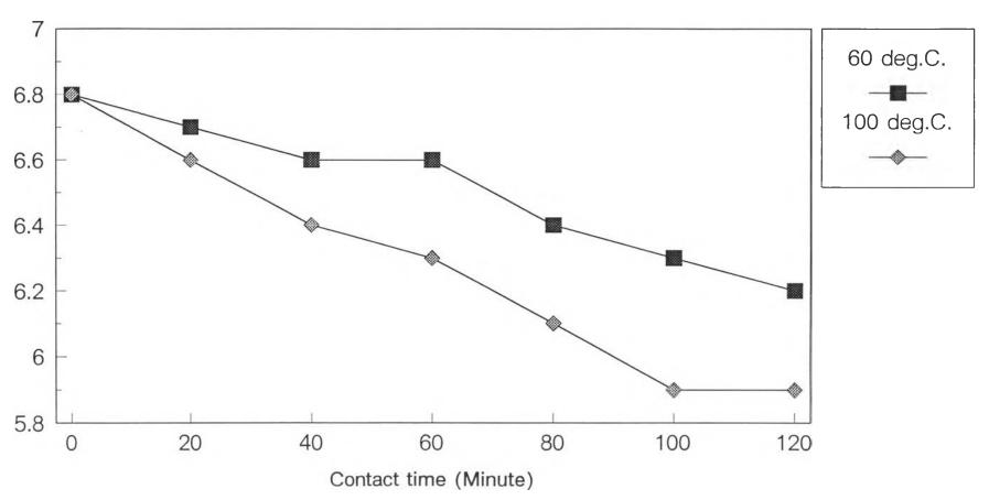
Fig. 5.17 Sulphur content of 600 SN after percolation process at various contact and different temperature, 60 C. and 100 C.
