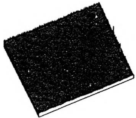
Figure 26 Optical Microscopic images of BPDA/PPD coated on Si<100> wafer cured at 400°C for 30 minutes.
