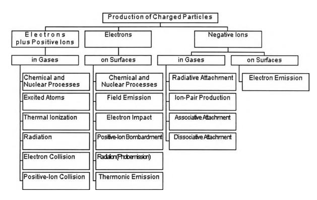
Figure 2.1 The alternative methods of charged particles generation.
