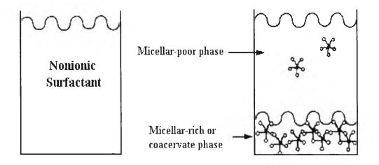
Figure 2.4 Schematic diagram of phase separation in nonionic surfactant.
