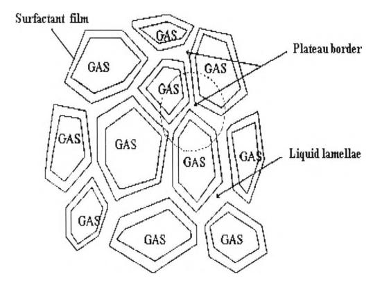
Figure 2.3 The structure of foam.
