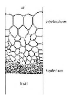
Figure 2.4 The two types of foam : polyederschaum, kugelschaum.
