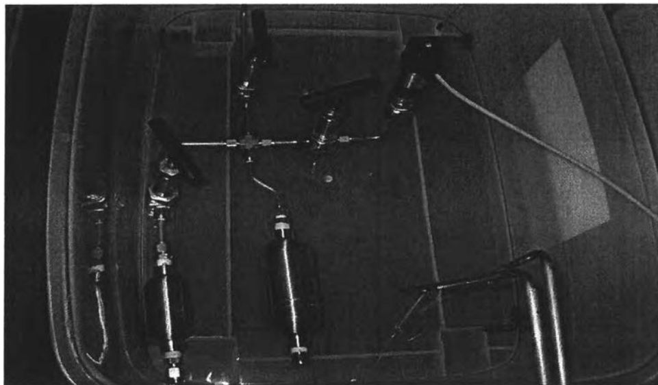
Figure 3.4 The constant volumetric isothermal adsorption apparatus.
