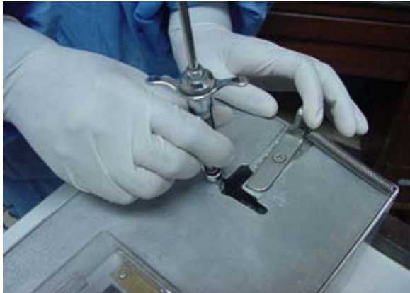
Figure 5. Shows the loosened needle can be removed by a gentle force.
