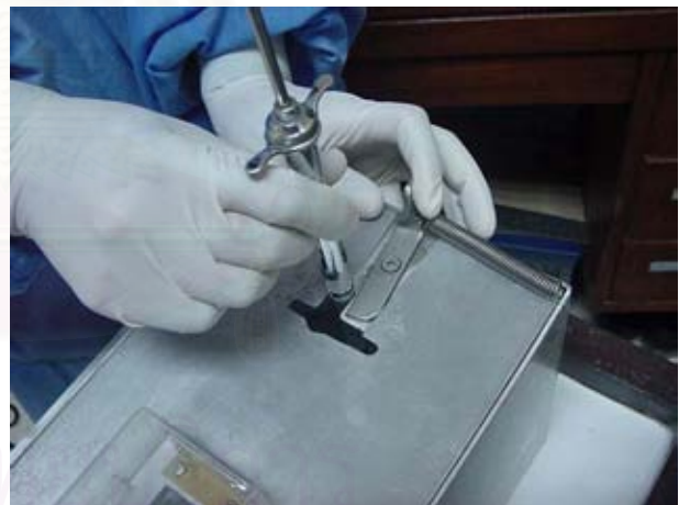
Figure 4. Shows the screw needle is fixed by a serrated end hinge which was fixed by a sided spring.
