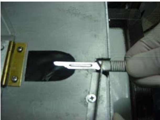
Figure 2. Shows the moved hinge is served the raised blade and pulling the handle of the blade out.
