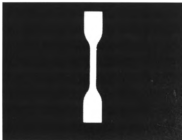
Figure 3.2 Dumbbell specimen for tensile test.
