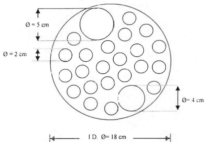
**Figure 3.2** Schematic of tray (Top view).
