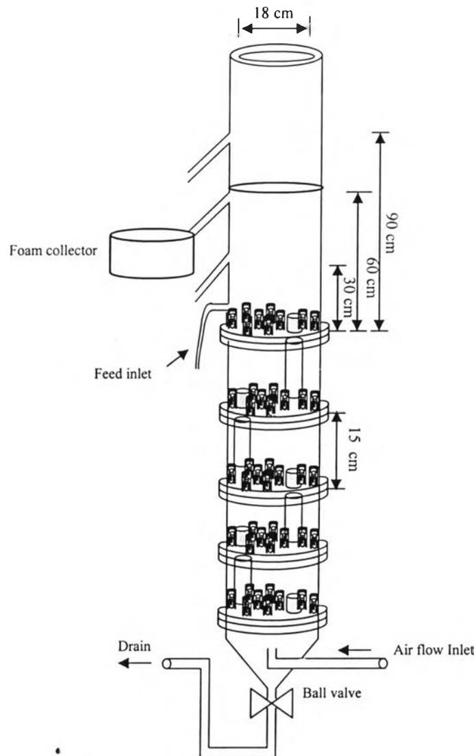
**Figure 3.1** Schematic of multistage foam fractionation column.
