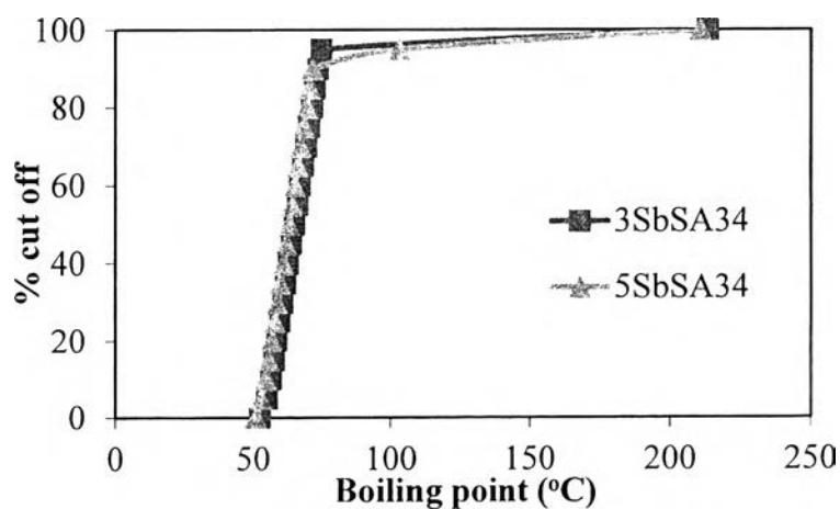
**Table E5** True boiling point curves of oil from using KOH-treated HZSM-5 catalysts
