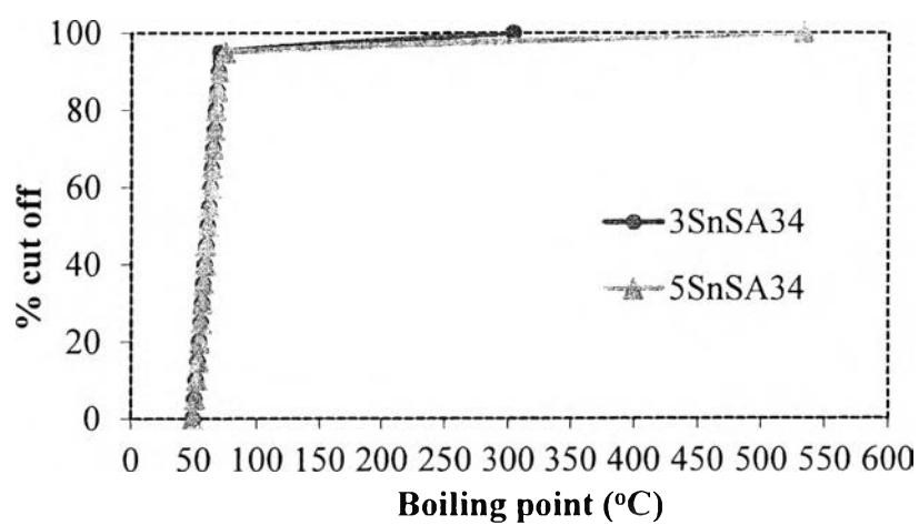
**Table E4** True boiling point curves of oil from using antimony oxide-doped SAPO-34 as a catalyst
