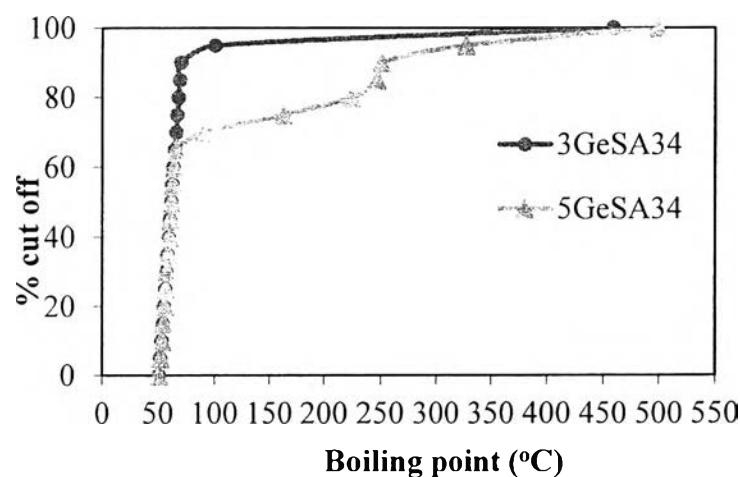
**Table E2** True boiling point curves of oil from using gallium oxide-doped SAPO-34 as a catalyst
