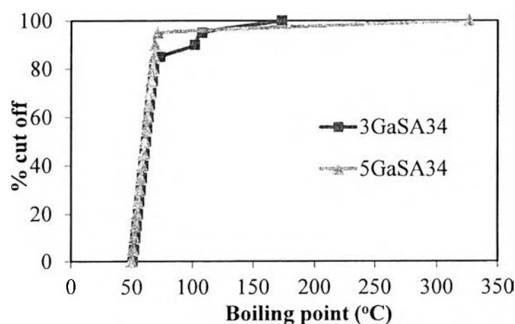
**Table E3** True boiling point curves of oil from using tin oxide-doped SAPO-34 as a catalyst
