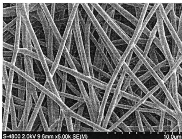
Figure 4.1 Selected SEM image of PCL electrospun fibrous scaffolds (magnification = 5000x; scale bar = 10 \mu\text{m} ).
