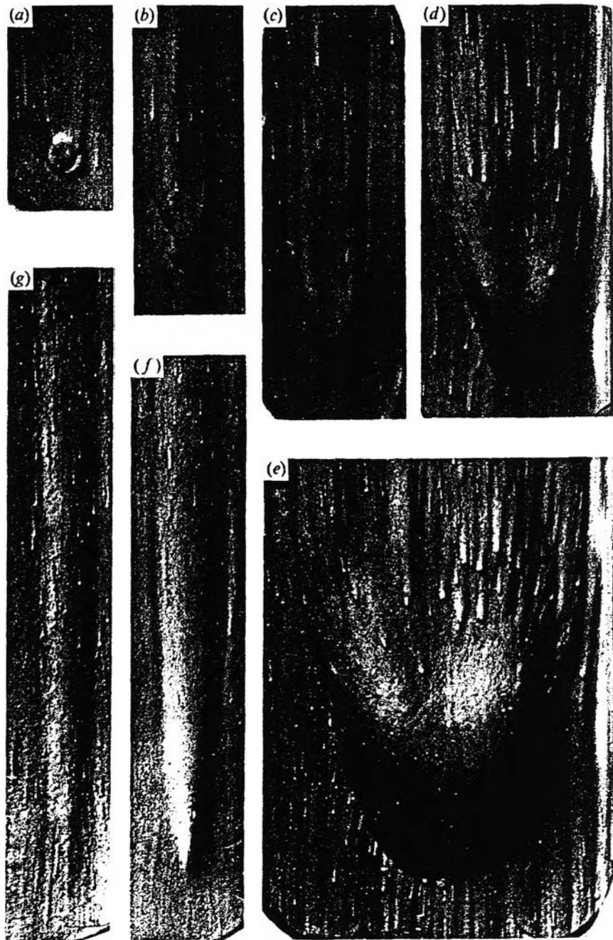
Figure 2.4 Stages in the development of experimental Flutes (a-e) and grooves (f), (g) from defects introduced into Plaster of Paris beds. Flow from bottom to top. (e) is 10 cm wide. (Allen, 1971)
