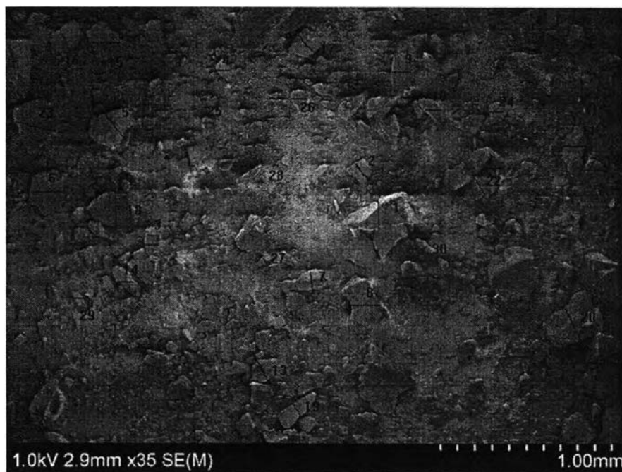
Figure E-4 Particle of Dai coal after grinding from SEM.
