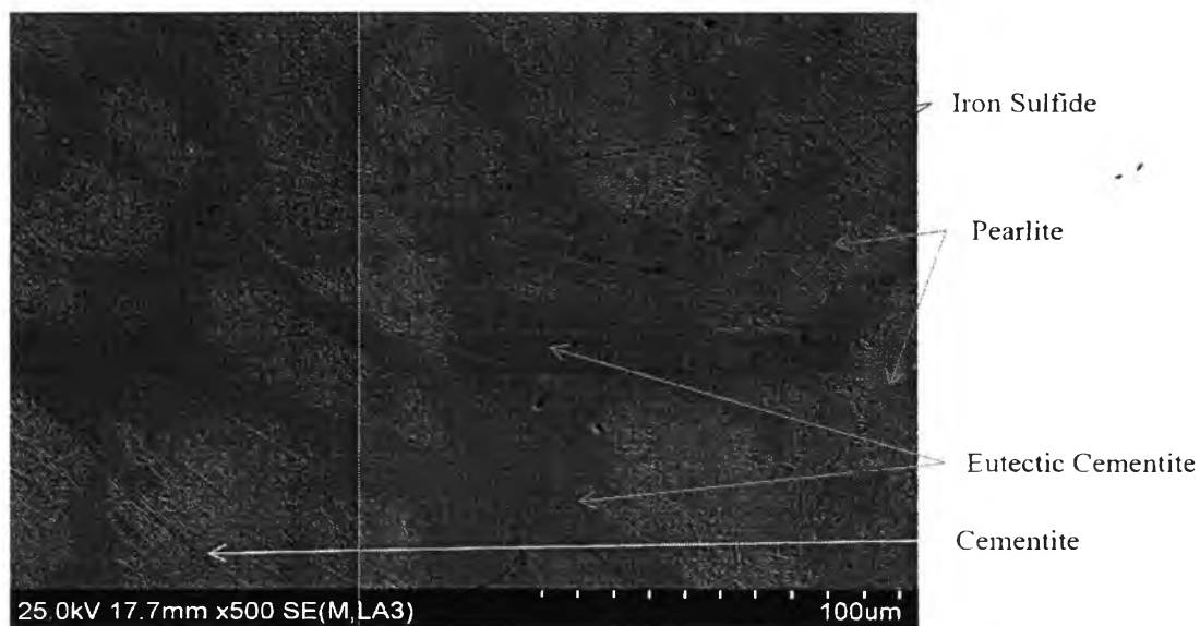
Figure E-5 The backscattered SEM image of cross section iron nugget from Experiment 6, No. 3 at reduction temperature 1,425°C and reduction time of 20 min.
