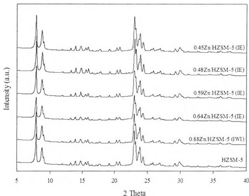
**Figure 4.5** XRD patterns of HZSM-5 and Zn/HZSM-5 zeolites prepared by aqueous phase ion-exchange (IE) and incipient wetness impregnation (IWI) methods.
