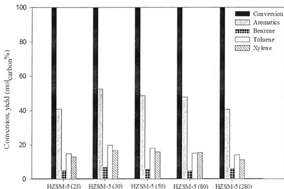
**Figure 4.3** Effect of  $\text{SiO}_2/\text{Al}_2\text{O}_3$  ratios of HZSM-5 zeolite on the glycerol conversion and aromatics yield. Reaction conditions: 300 psig, 400 °C, WHSV = 1  $\text{h}^{-1}$ , and TOS = 3 h.
