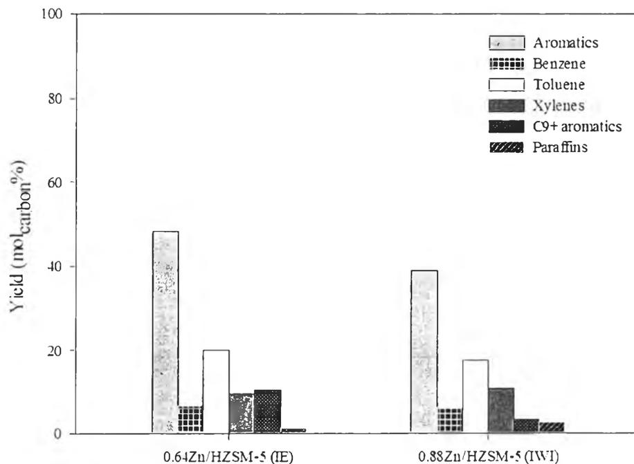
**Figure 4.14** Glycerol conversion and aromatics yield as a function of preparation methods, 0.64Zn/HZSM-5 (IE) and 0.88Zn/HZSM-5 (IWI). Reaction conditions: 300 psig, 400 °C, WHSV = 3.33 h<sup>-1</sup>, and TOS = 3 h.
