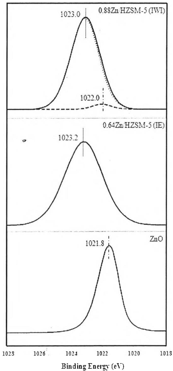
**Figure 4.9** XPS spectra of Zn (2p<sub>3/2</sub>) of 0.88Zn/HZSM-5 (IWI), 0.64Zn/HZSM-5 (IE), and ZnO.
