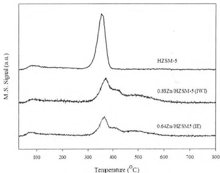
**Figure 4.7** Isopropylamine-TPD (IPA-TPD) profiles of Zn/HZSM-5 prepared by incipient wetness impregnation (0.88Zn/HZSM-5 (IWI)) and aqueous phase ion-exchange methods (0.64Zn/HZSM-5 (IE)). The mass monitored was propylene ( $m/e = 41$ ).
