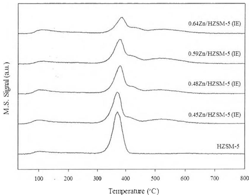
**Figure 4.6** Isopropylamine-TPD (IPA-TPD) profiles of parent HZSM-5 and Zn/HZSM-5 (IE). The mass monitored was propylene ( $m/e = 41$ ).
