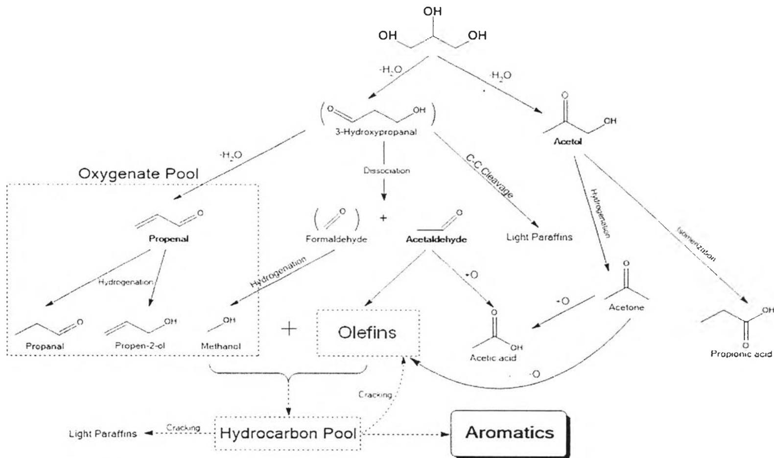
Figure 4.2 Proposed reaction pathway for converting glycerol to aromatics.
