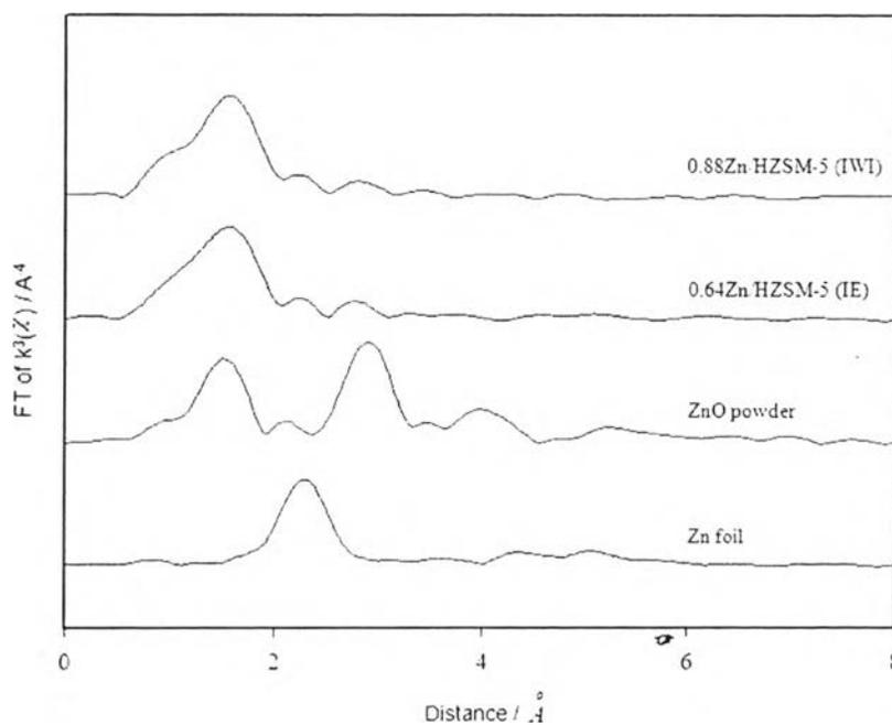
**Figure 4.10** EXAFS of Zn K-edge radial distributions of 0.64Zn/HZSM-5 (IE), 0.88Zn/HZSM-5 (IWI), ZnO powder, and metallic Zn foil.
