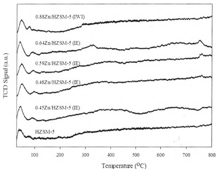
**Figure 4.11** Temperature programmed reduction (TPR) profiles of 0.88Zn/HZSM-5 (IWI), 0.64Zn/HZSM-5 (IE), 0.59Zn/HZSM-5 (IE), 0.48Zn/HZSM-5 (IE), 0.45Zn/HZSM-5 (IE), and HZSM-5.
