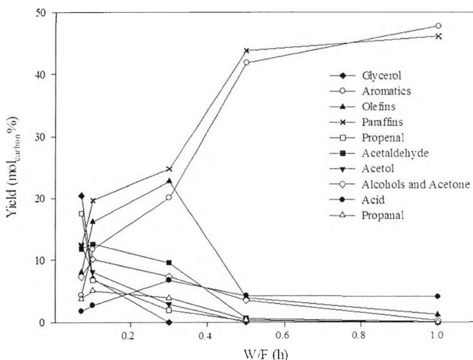
**Figure 4.1** Product yield of glycerol conversion over HZSM-5 with  $SiO_2/Al_2O_3$  ratio of 80 as a function of space time (W/F). Reaction conditions: 300 psig, 400 °C, and TOS = 3 h.
