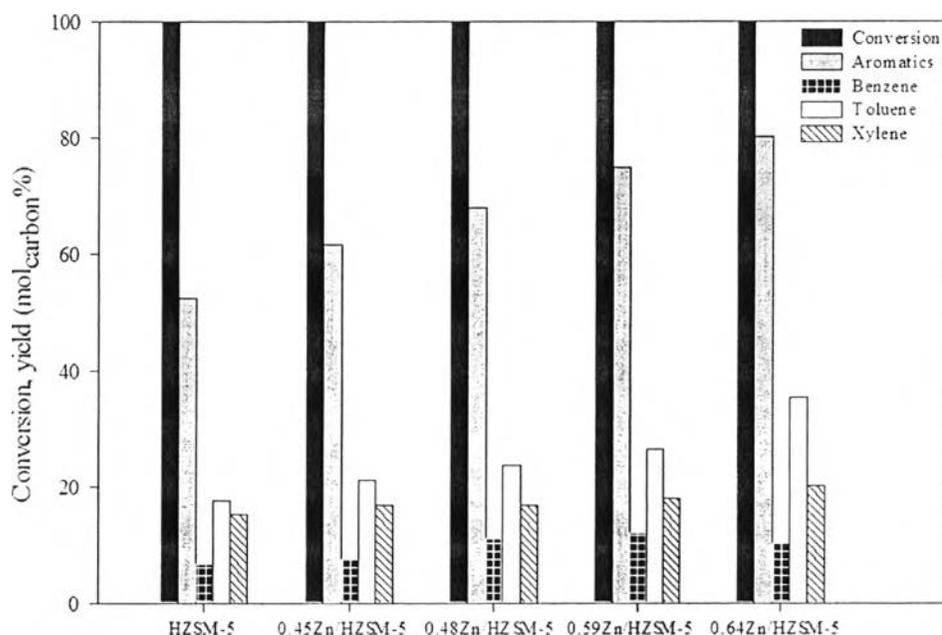
**Figure 4.12** Glycerol conversion and aromatics yield as a function of Zn loading by aqueous phase ion-exchange (IE) method. Reaction conditions: 300 psig, 400 °C, WHSV = 1 h<sup>-1</sup>, and TOS = 3 h.
