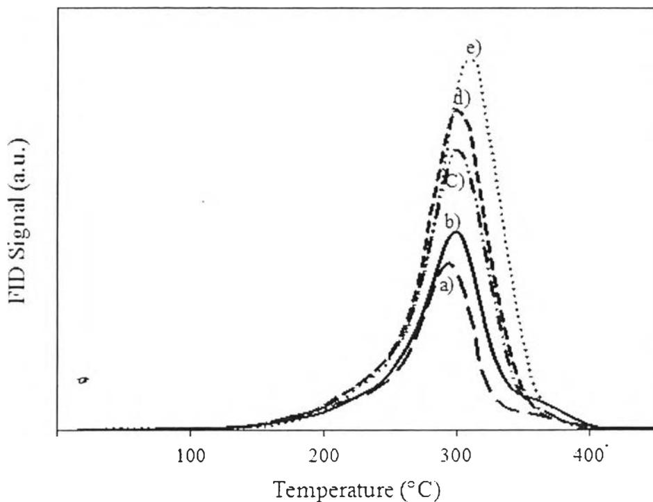
**Figure 4.4** TPO profiles of spent HZSM-5 with  $\text{SiO}_2/\text{Al}_2\text{O}_3$  ratios of a) 280, b) 23, c) 80, d) 50, and e) 30.
