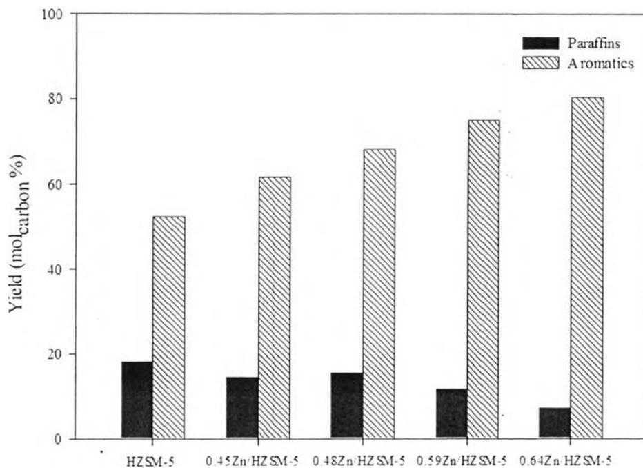
**Figure 4.13** The relationship between aromatics and light paraffins yields as a function of Zn loading by aqueous phase ion-exchange (IE) method. Reaction conditions: 300 psig, 400 °C, WHSV = 1 h<sup>-1</sup>, and TOS = 3 h.
