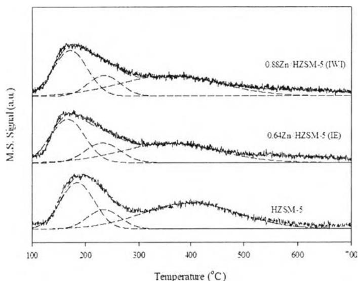
**Figure 4.8** Ammonia-TPD ( $\text{NH}_3$ -TPD) profiles of Zn/HZSM-5 prepared by incipient wetness impregnation (0.88Zn/HZSM-5 (IWI)) and aqueous phase ion-exchange methods (0.64Zn/HZSM-5 (IE)). The mass monitored was ammonia ( $m/e = 17$ ).
