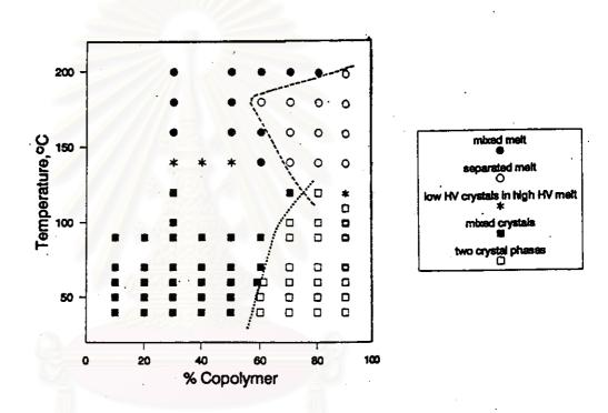
Figure 2-3 Summary of DSC results. The dashed curve (----) shows approximate position of the boundary for liquid-liquid phase separation. The dotted curve (.......) shows the boundary between single-two phase crystallization [Organ and Barham, 1993].
