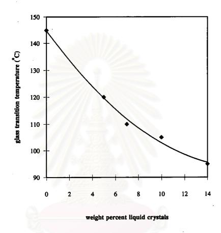
**Pigure 2-2** Glass transition temperature depression in blends of bisphenol-A-polycarbonate and p-pentyloxycinnamic acid [Patwardhan and Belfiore, 1988].
