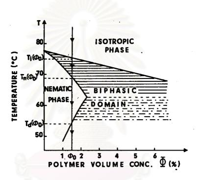
Figure 2-1 A typical phase diagram of flexible polymer in nematic solvent
