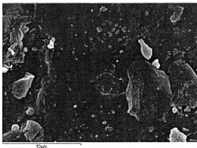
Figure 2.7 SEM micrograph of natural rubber latex/chitosan blends.
