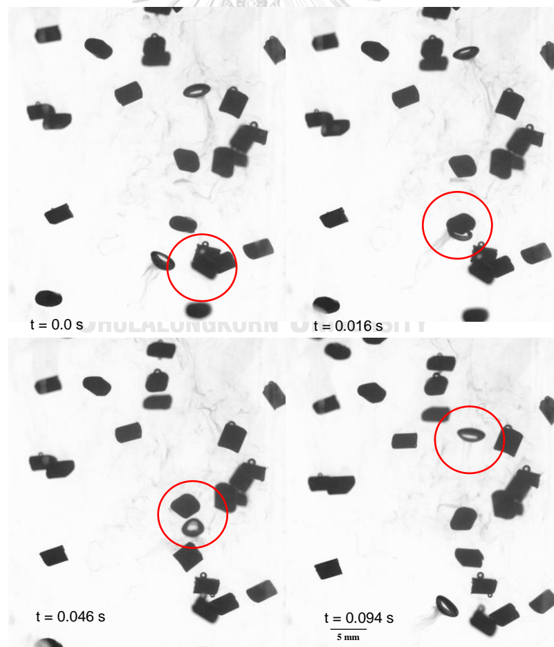
Figure 4.21 Trajectory of a small bubble with a collision with a particle and its oxygen transferred regime
