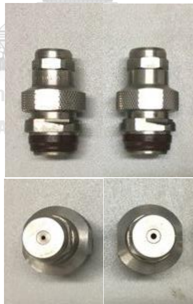
Figure 2.4 Full-cone spray nozzles (left) 0.89 mm (right) 1.50 mm
