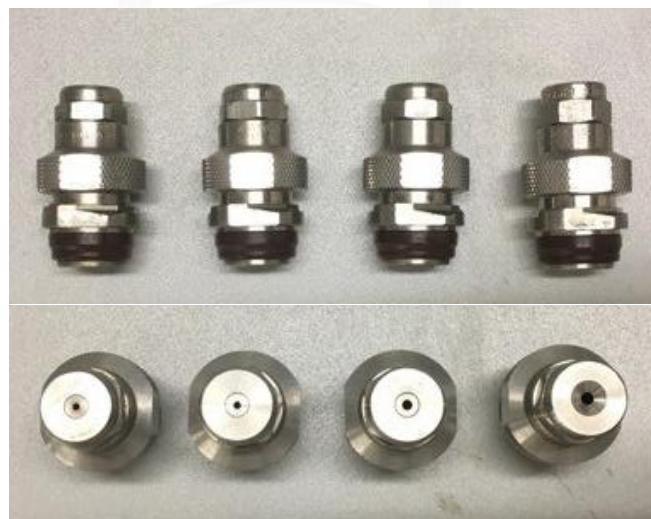
Figure 3.4 Full cone spray nozzle at different orifice sizes (Left to right) 0.89 mm, 1.20 mm, 1.50 mm, and 2.00 mm
