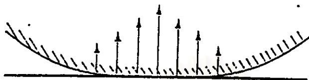
Pressure Distribution Around the Contact Area When a Floc is at Rest on a Solid Plane (Yusa, Suzuki and Tanaka, 1975)
