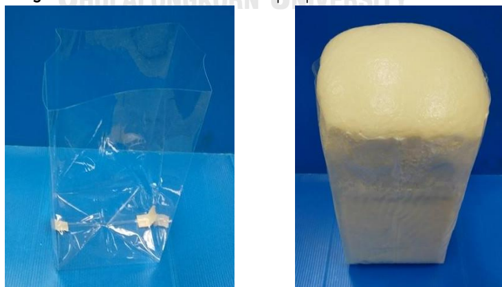
Figure 3.2 Plastic bag for used in molded method
