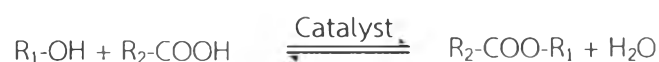
Figure 2.14 General esterification of carboxylic acid with alcohol in the presence of catalyst.
