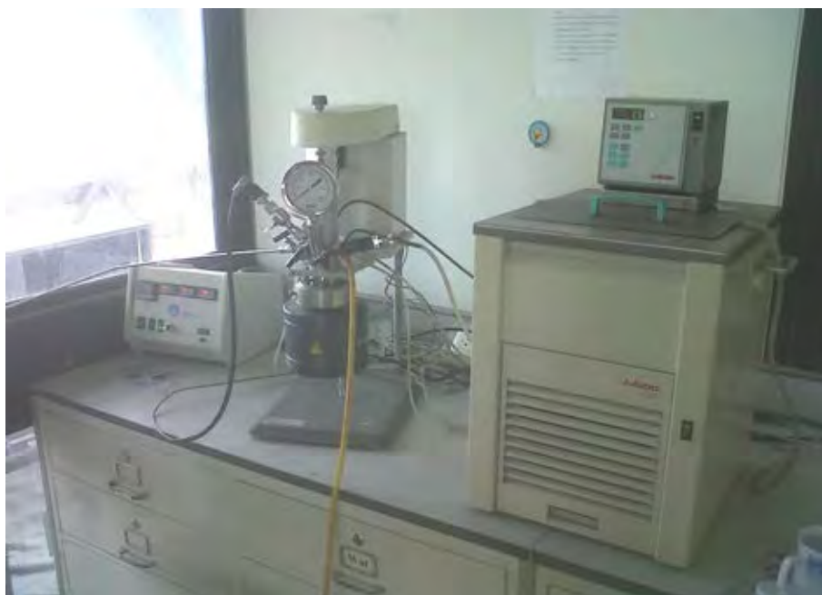
Figure 3.1 Schematic of the experimental setup for the utilizing CO 2 of amine, butyl bromide, using Parr reactor, PBTR.
