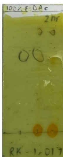
Figure 30: TLC of the reaction after ozonolysis for 2 hours under 2,4-DNP staining agent
