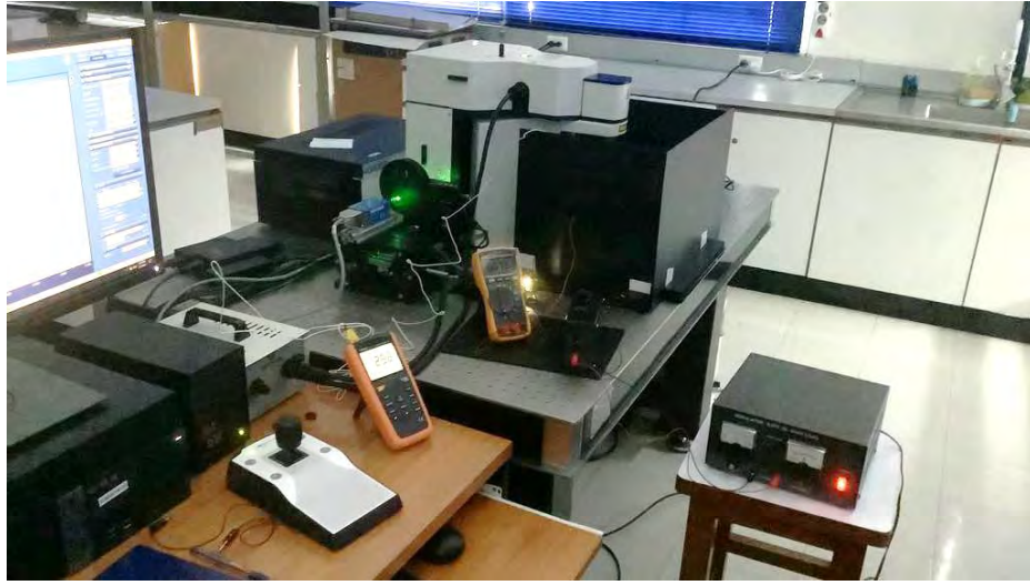
Fig 28. Temperature-dependent Raman setup.
