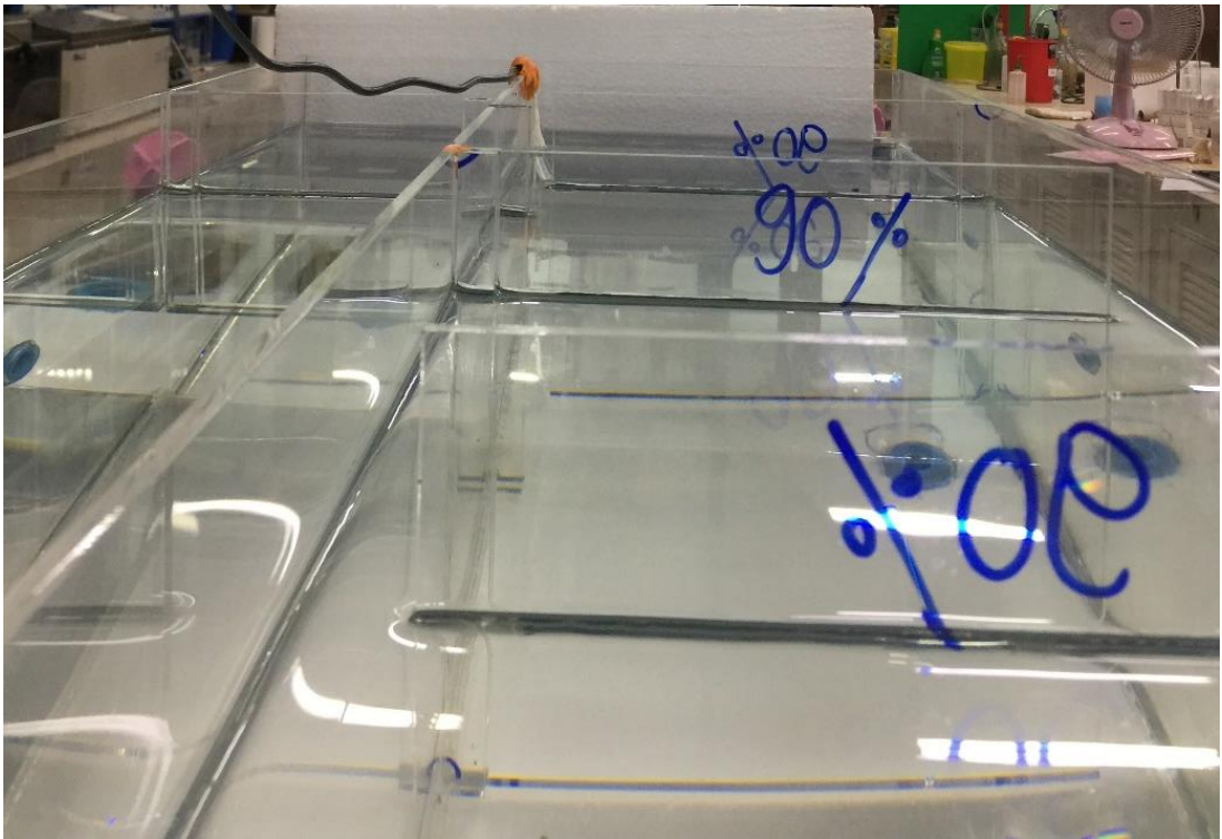
Figure 8. The experiment of RTD methods on effect of baffles
