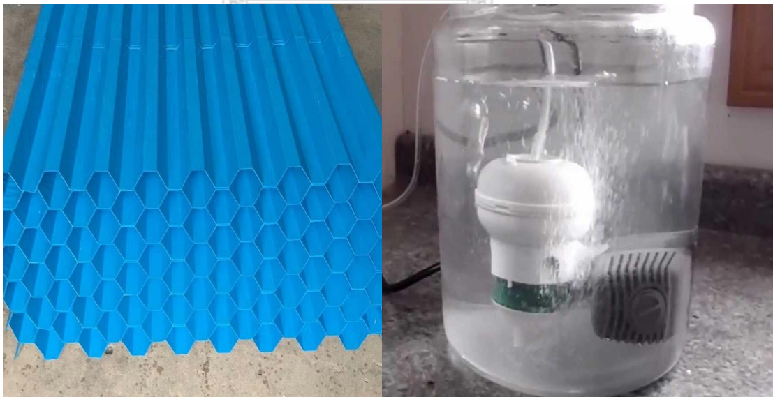
Figure 2.8. Equipment of improvement separation: plate and tube settler (left), micro bubble generation (right)
