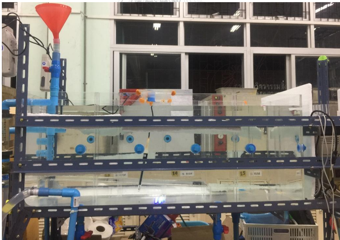
Figure 7. The experiment of RTD methods on effect of probe position
