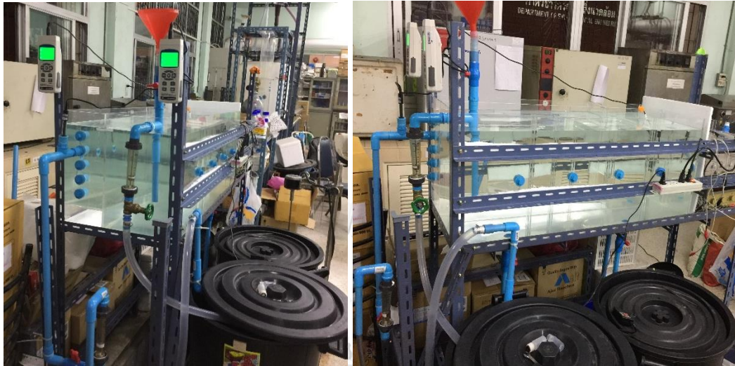
Figure 6. The experiment of RTD methods on ECR reactor without any conditions\
