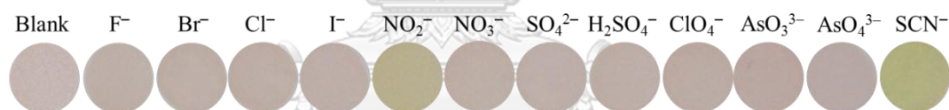
Figure 4.33 Colors of paper-based optode with the L3 toward different 1 mM of anions in 0.01 M tris-HCl buffer solution at pH 7.4 with the immersing time of 15 minutes.
