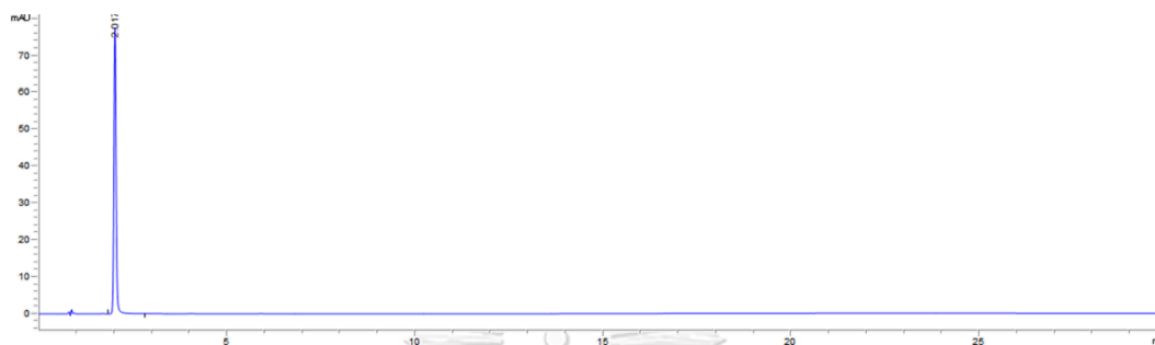
Figure 40 HPLC chromatogram of OXY standard with retention time at 2.0 min. The detection was measured at 320 nm.
