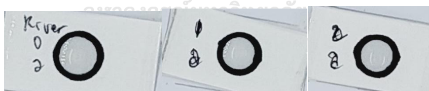
Figure 33. Spike river water before filtration with 0 (non-spiked); 1 (10 \mu\text{g/L} ); 2 (20 \mu\text{g/L} )
