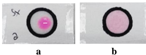
Figure 13. The comparison of final solution color intensity in (a) pre-wetted paper platform and (b) normal paper platform
