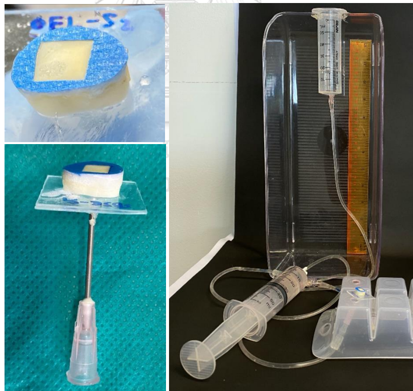
Figure 3 Tooth preparation and simulated fluid flow through a sectioned crown using 20 cm distilled water pressure
