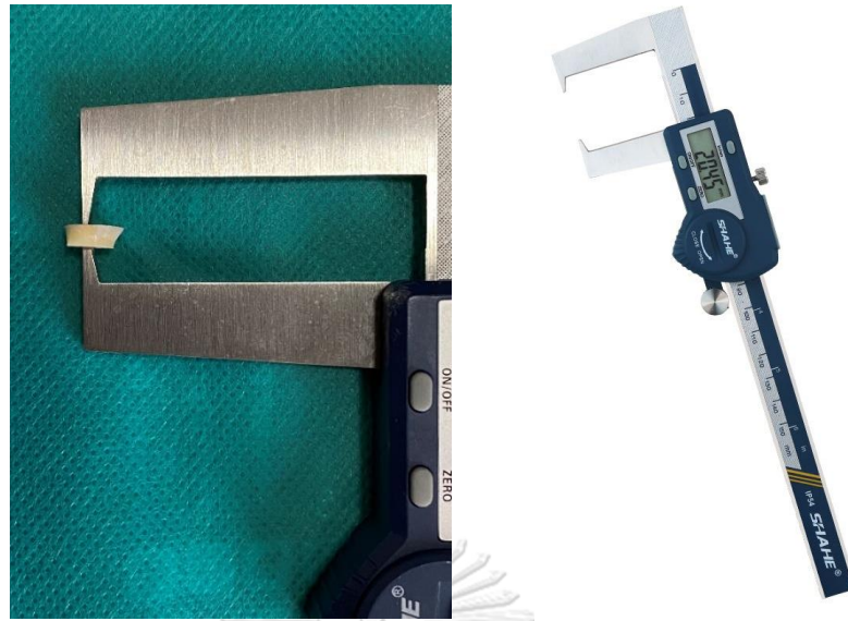
Figure 2 Remaining dentin thickness was confirmed by a digital vernier caliper (SHAHE, China).
