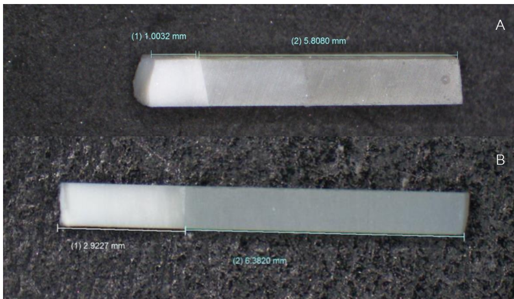
Figure 6 The resin-dentin stick used for microtensile test
