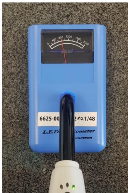
Figure 4 Light-curing unit with > 600 \text{ mW/cm}^2 intensity was checked with a Radiometer (L.E.D. radiometer by Demetron, Kerr Corporation, Danbury, CT, USA)
