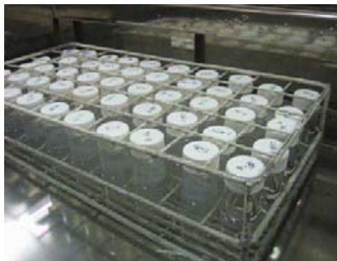
Figure 3.3 Surfactants equilibrated in water bath to induce the phase separation
