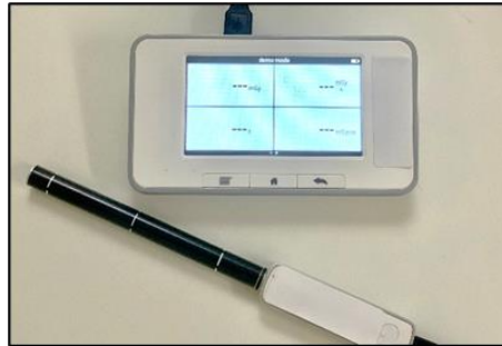
Figure 4.2: Pencil-type ionization chamber RaySafe X2 CT Detector and the electrometer
