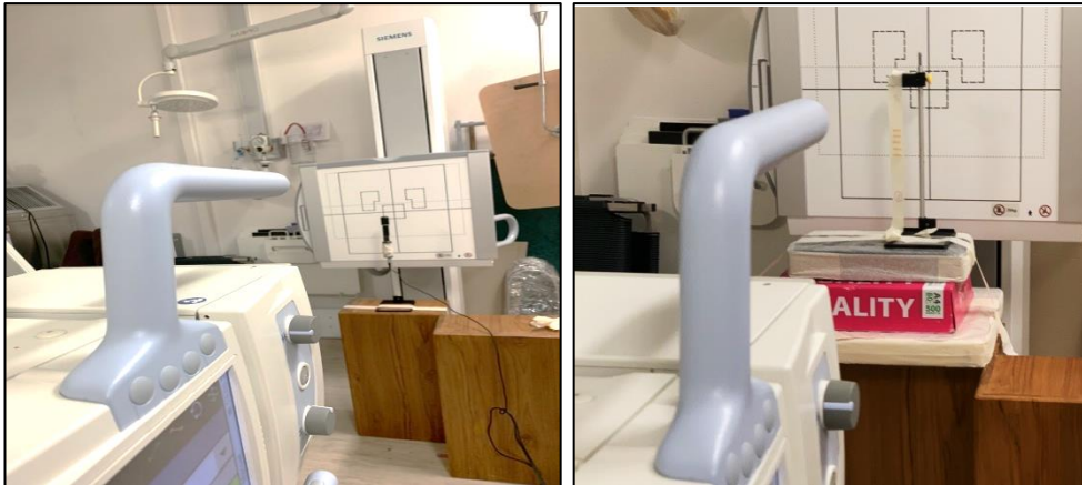
Figure 4.11: Set the SDD for the ionization chamber and RPLGDs at 150 cm for the calibration.
