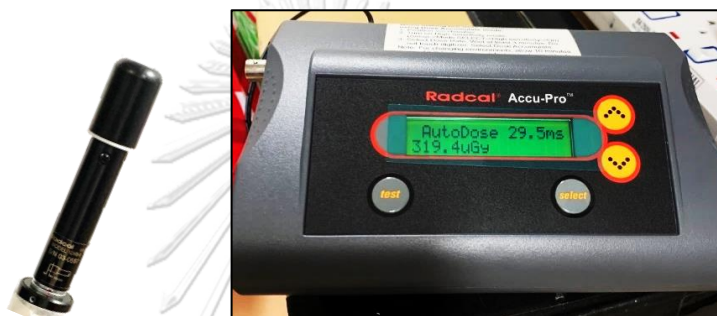
Figure 4.6: A 6-cc ion chamber Model 10X6-6 and Radcal 9096 electrometer (Radcal, Monrovia, CA, USA)
