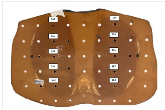
Figure 6.1: RPLGDs were inserted into the holes along the central axis of the lungs.
