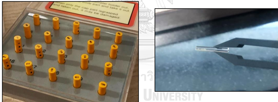
Figure 4.3: Radio-photoluminescence Glass Dosimeter (RPLGD), model GD-352M with filters in capsule (Left), Glass rod (Right)
