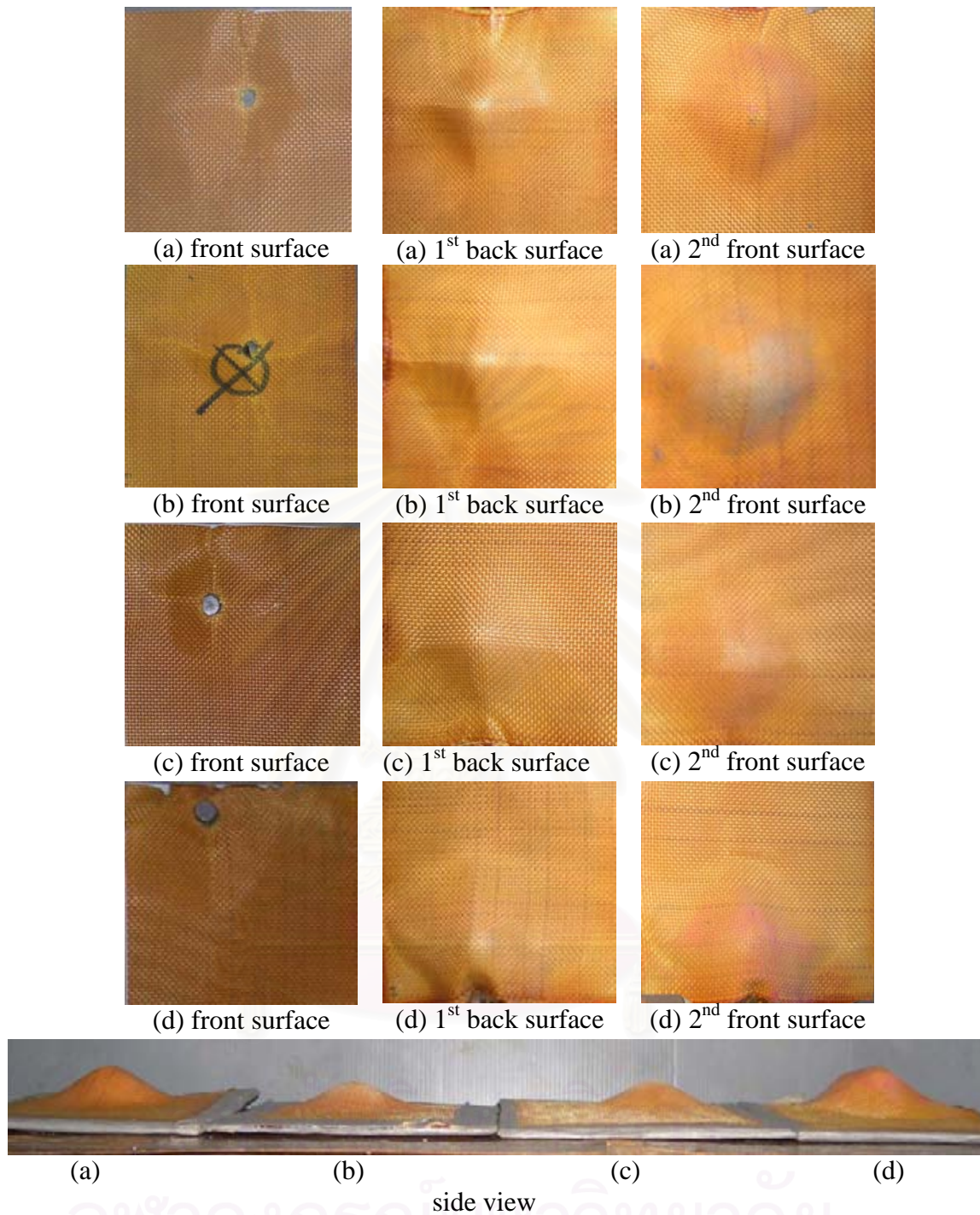
Figure 5.47: Damaged and delaminated area of 5 piles/panel with the samples arrangement of 5/5 after impact with standard lead projectiles with lead outer-coating typically used in 9 mm: (a) Kevlar TM -reinforced 80:20 BA:PU1K, (b) Kevlar TM reinforced 80:20 BA:PU2K, (c) Kevlar TM -reinforced 80:20 BA:PU3K, and (d) Kevlar TM -reinforced 80:20 BA:PU5K
