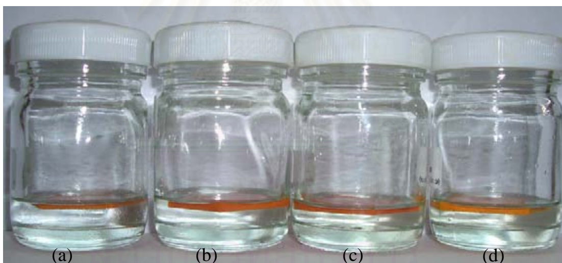
Figure 5.44: The Polymer Alloys Specimens (BA:PU=80:20) Immersed in Chloroform for 30 days : (a) MW 1000, (b) MW 2000, (c) MW 3000, and (d) MW 5000
