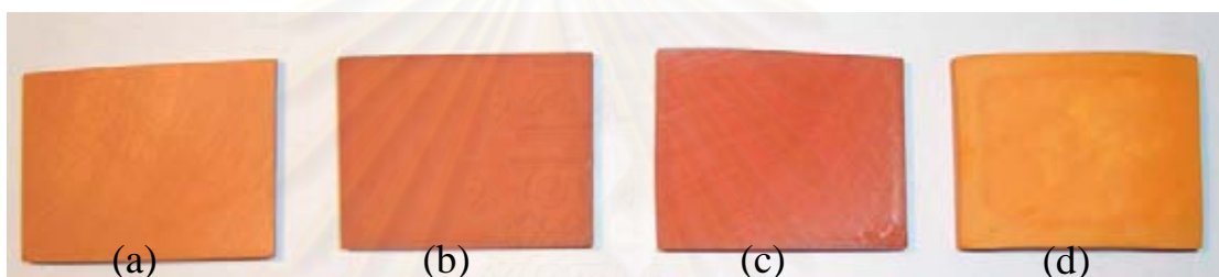
Figure 5.38: The Polymer Alloys Specimens (BA:PU = 80:20) after Immerse in Chloroform: (a) MW 1000, (b) MW 2000, (c) MW 3000, and (d) MW 5000
