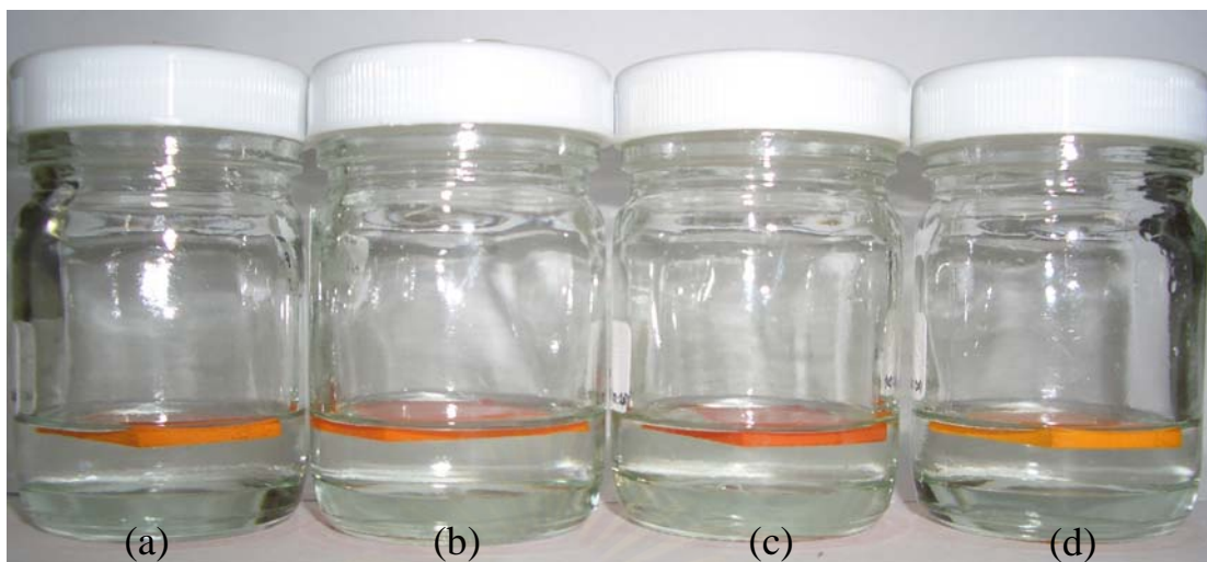
Figure 5.43: The Polymer Alloys Specimens (BA:PU=80:20) Immersed in Chloroform for 14 days : (a) MW 1000, (b) MW 2000, (c) MW 3000, and (d) MW 5000
