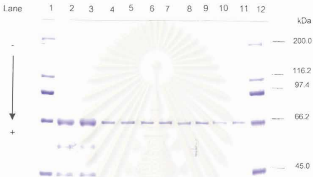
Figure 22. SDS-PAGE of CGTase treated with TFMS
