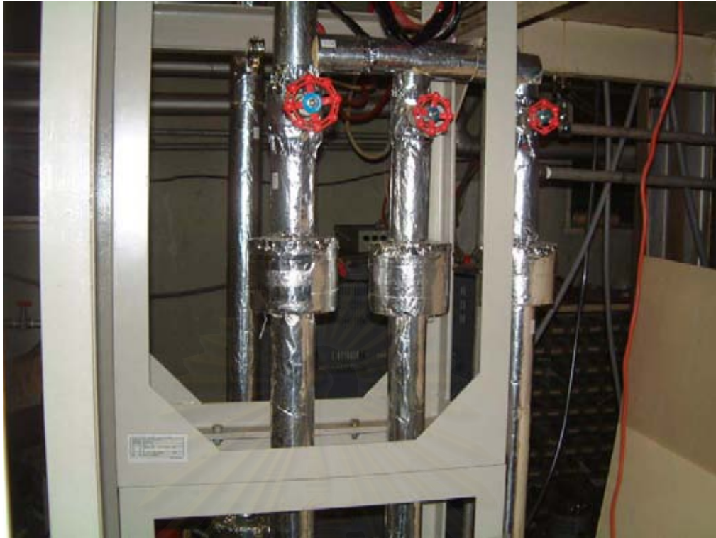
Fig.4.2 three parallel channels with high-, medium-, and low-range orifices
