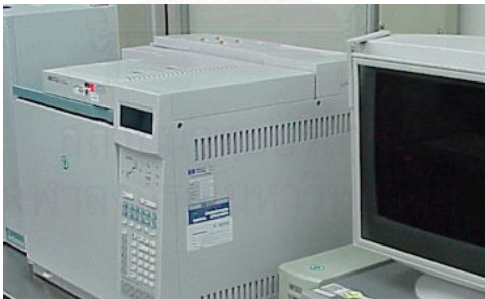
Figure 3.2 Gas Chromatography (instrument for measure light oil in water)
