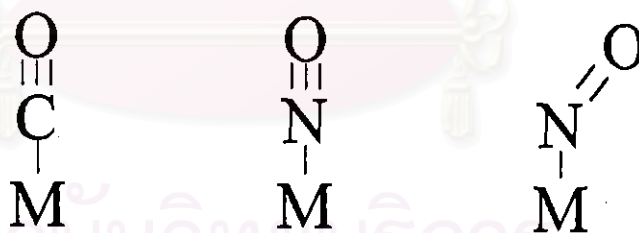
Figure 3.3 The adsorption of CO and NO on catalyst surfaces
