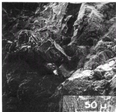
Fig. 2.12 SEM micrograph of the surface of a broken briquette : size and shape of flue-gas gypsum particles have disappeared.
