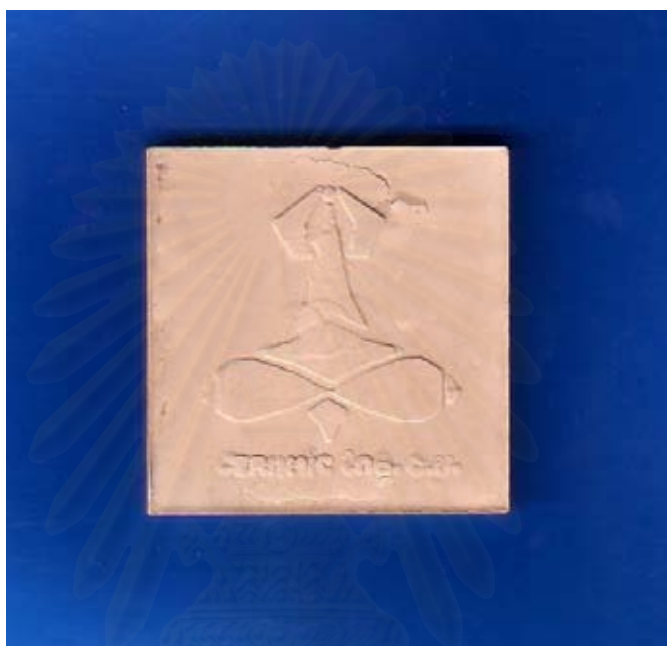
Fig. 4.10 FGD briquette pressed at 180 bars.
