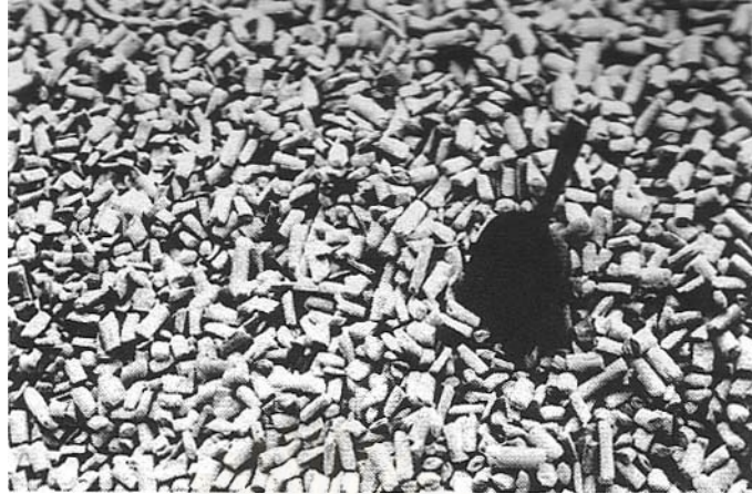
Fig. 2.8 Flue-gas gypsum briquettes in storage.
